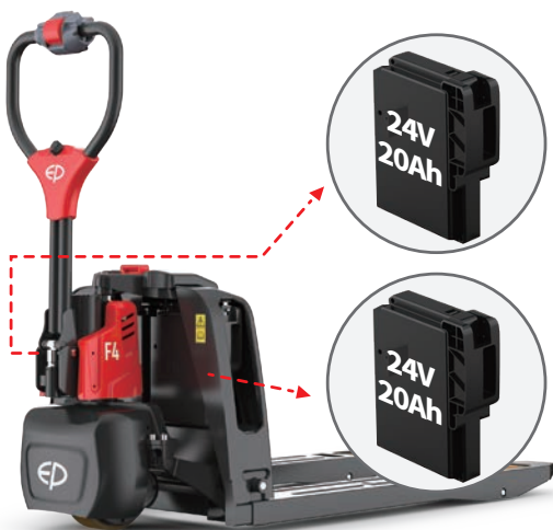
Heavy-duty Estimated real life working time: 11hrs
